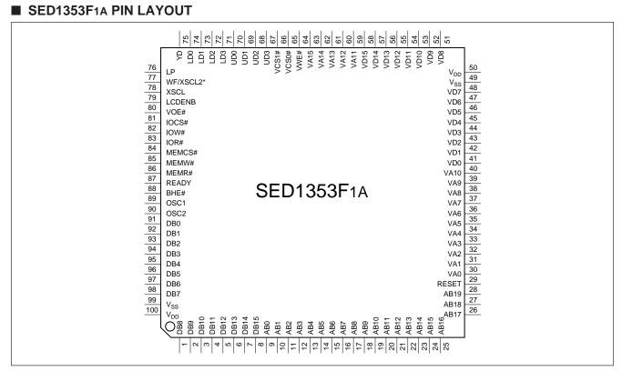
\* Pin No. 77 = WF: Supports every display mode except for 8-bit single color panel interface (format 1).
