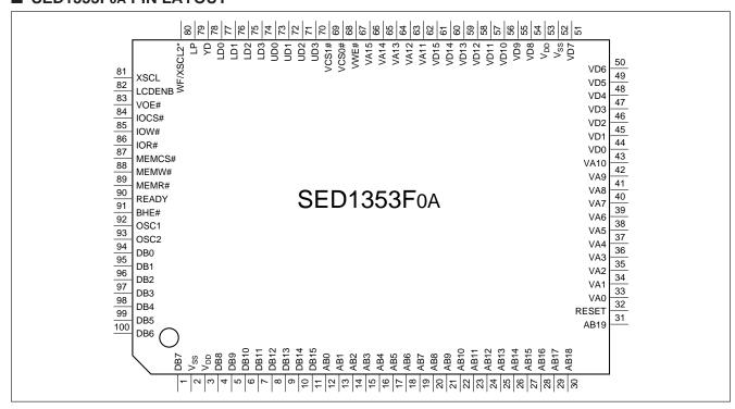
\* Pin No.80 = WF: Supports every display mode except for 8-bit single color panel interface (format 1).
