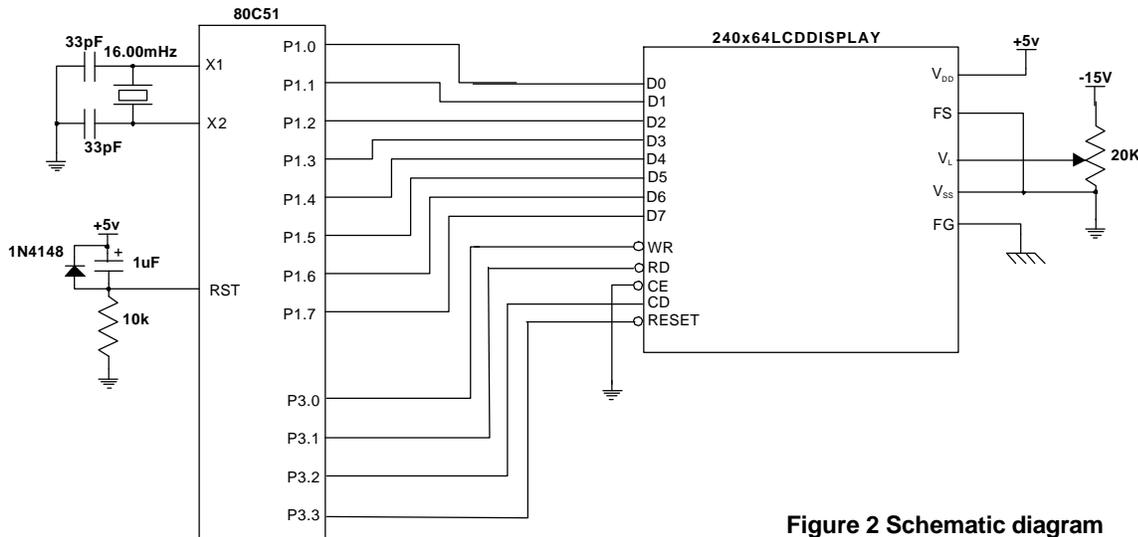
Figure 2 Schematic diagram
